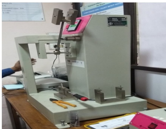
Fig 7: Izod impact test experimental setup
