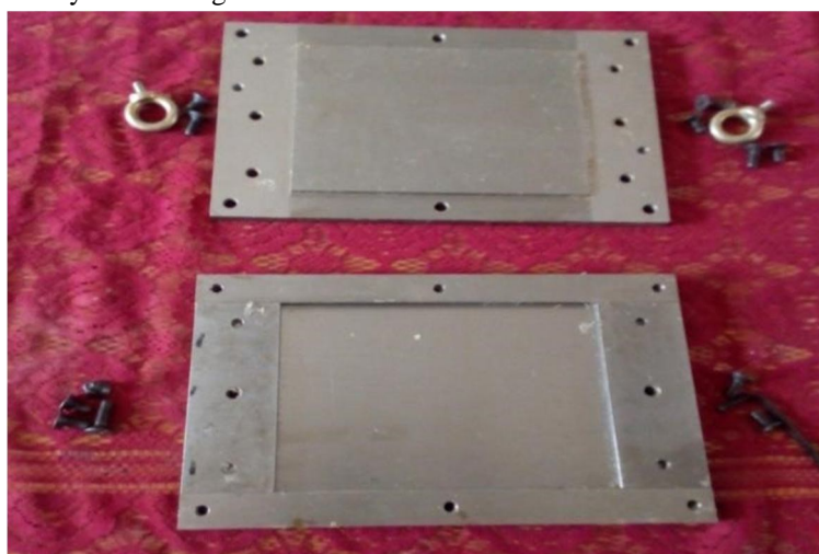
Fig 4: Mold used for hand layup
