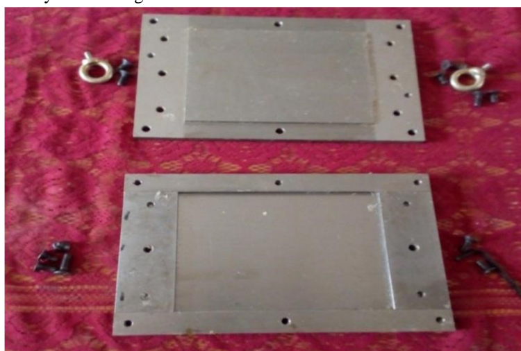
Fig 4: Mold used for hand layup
