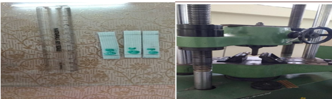
Fig 6: 3-point bending test specimen and experimental setup
