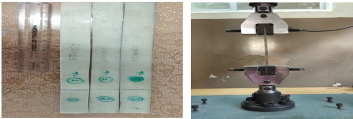
Fig 5: Tensile test specimen and experimental setup
