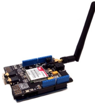
Fig 3. GPRS Shield Interfaced To Arduino Uno
