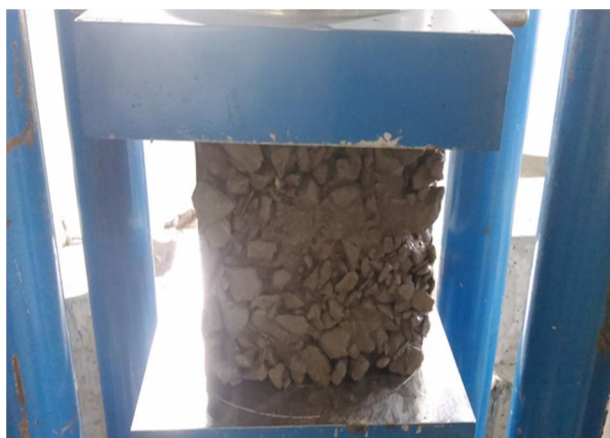
Fig.2: Cube Compressive strength test for prepared cube
