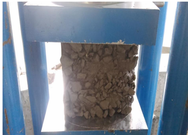
Fig.2: Cube Compressive strength test for prepared cube
