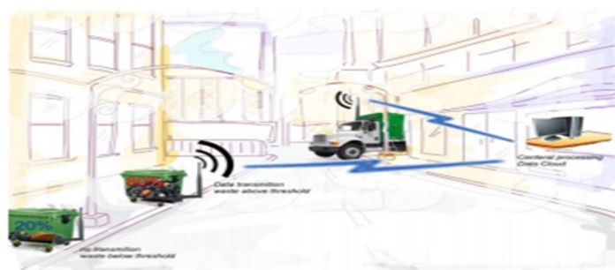
Fig. 1. A schematic of the proposed IoT-based waste management architecture, showing the interconnectivity between the smart bins, the collection vehicles and the cloud.
