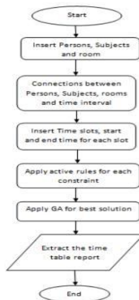
Block diagram of proposed architecture of automatic timetable generation.
