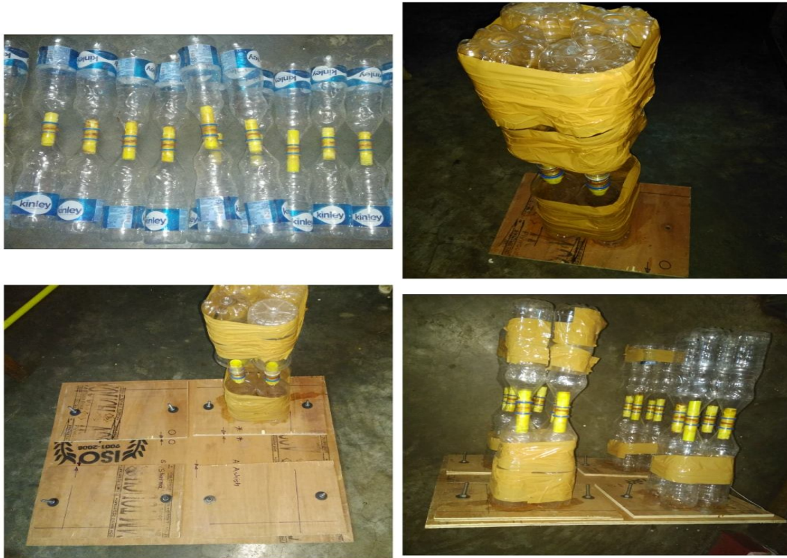
Fig. : Steps showing how we made leg from 4 connected bottles. And then 4 legs are made. Top of table is made from plywood sheet. Legs are detachable with help of Nut-Bolt assembly. In case of breaking, we can change that portion which increases its useful life span and reliability of product.
