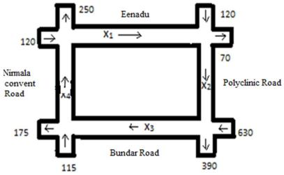
Consider the number of vehicles entering each intersection is equal to the number of vehicles leaving the intersection, this fact can be shown by an equation.
