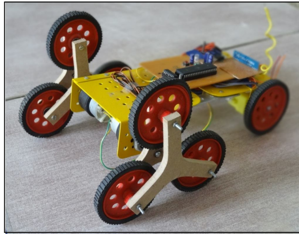
Fig.2: Wheel Structure and Frame of robot
