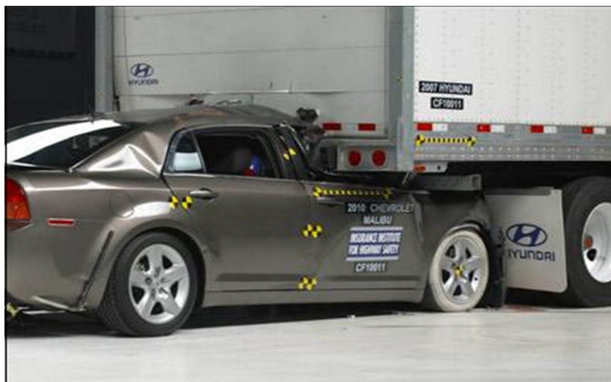
Fig. 1: Underride Crash of Car
