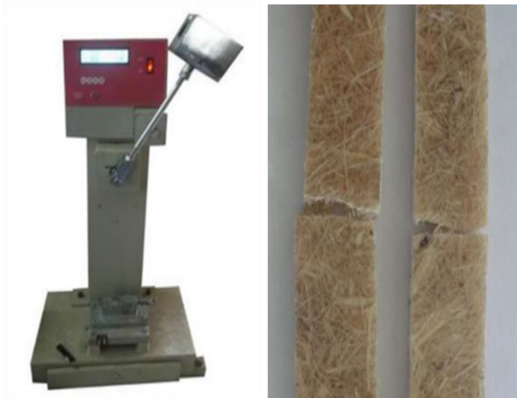
Fig.7. Impact Test Setup and Specimens.
