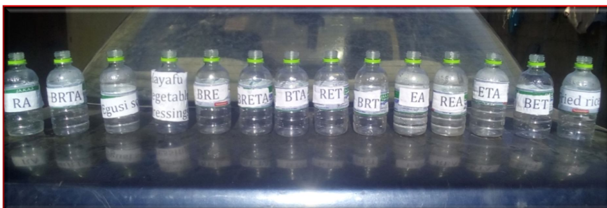
Plate VII: Coupons as soaked in the prepared menu media samples inside some containers in the laboratory with the identification labels
