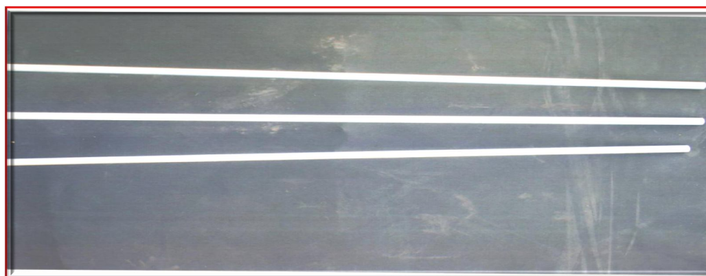
Plate II: The procured 6063 aluminum alloy rods used
