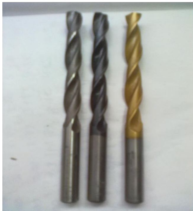
Figure4.1: HSS and coated TiN, TiAlN tools
