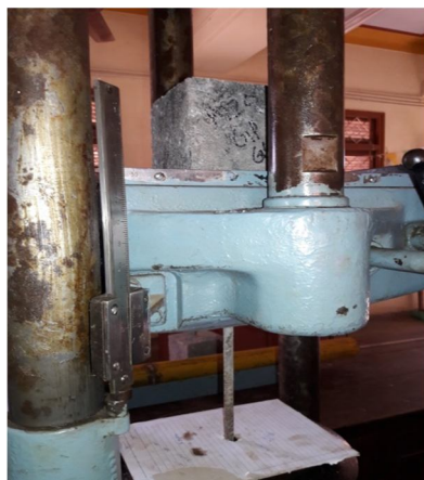
Figure 7. Pull Out Test Set up with specimen
