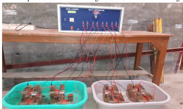
Figure 6. RCPT Test Set up with specimens
