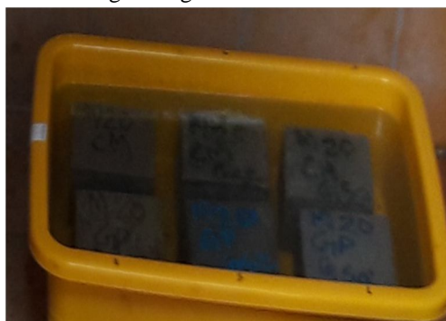
Figure 4. Specimens Immersed in H_2SO_4 Solution
