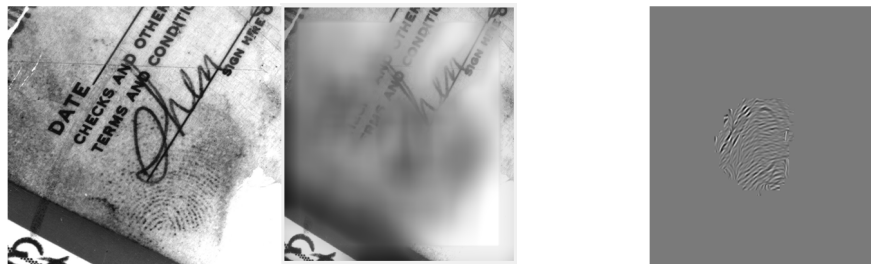
Fig 3 a) Original input image b) Output image of Wiener filter c) Output image of Gabor filter
