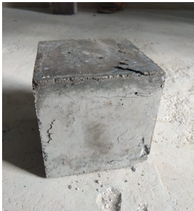
Fig.4 Cube Crack Pattern
