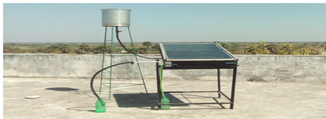
Fig 3 : Experiment setup without parabolic concentrator
