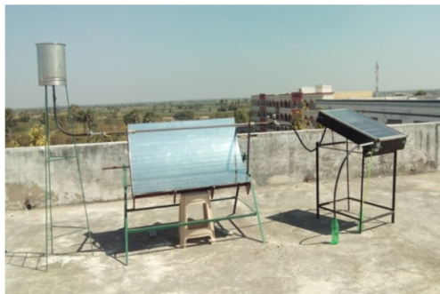
Fig 2: Experimental Setup of Stepped solar still with parabolic concentrator
