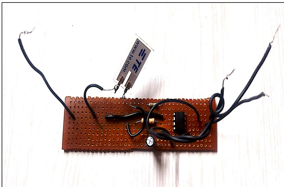
Fig. 6 Circuit of charge amplifier constructed by us
