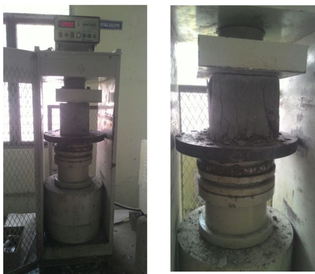
Fig 4.1. Test setup for Compressive strength of Cube
