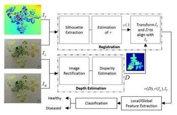
Once the image is captured the initial step will be a pre-processing step, it will process the image and removes voices to enhance it. It also includes enhancing the brightness for dim images. Silhouette extraction step enhances the shadow image to enhanced image by calculating the torque value and matches it with image that have high clarity. The leaves are classified as healthy and unhealthy leaves and their features are also extracted. This may train the system further better.
