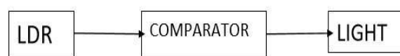
Fig. 2 – Block diagram which shows connection of LDR sensor, comparator and street light
