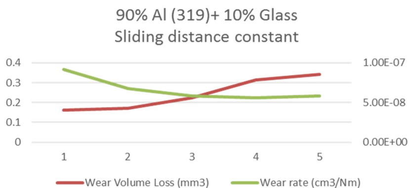
Fig.13 Wear rate of sample (90% Al + 10% Glass) sliding distance constant
