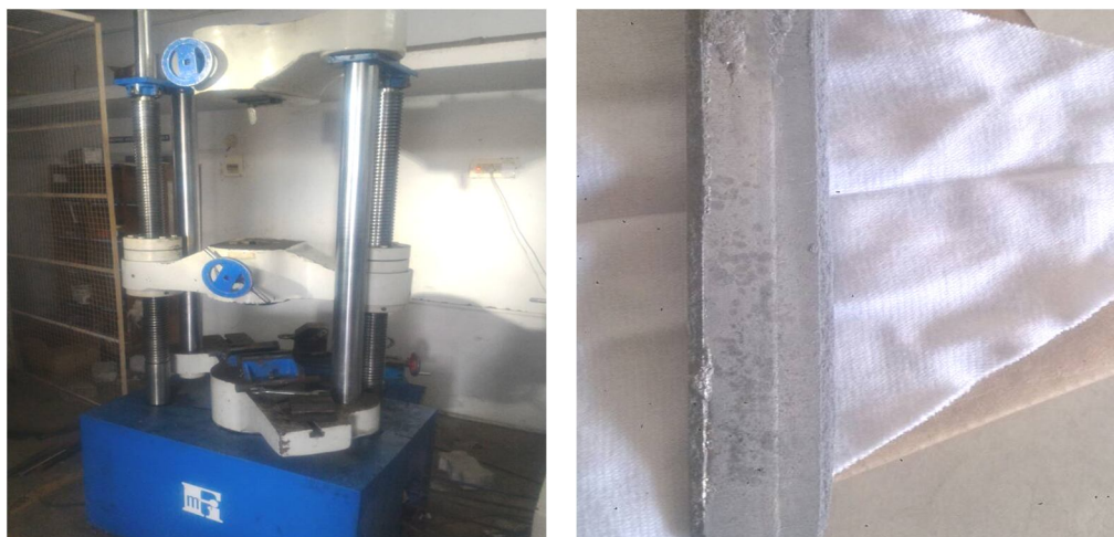
Fig.2 Universal machine & Tensile test specimen
