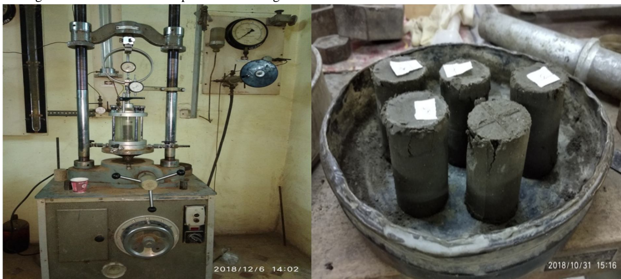
Figure2. Unconfined compressive strength test (UCS)
