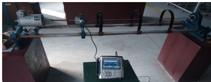
Fig. 2: Test Rig with Two End Fixed Support Bearings
