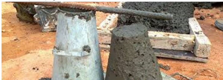
Fig 3.10 Testing for concrete workability
