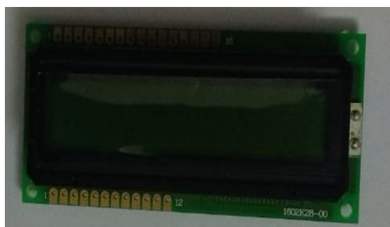
Figure 8: 16x2 LCD Display
