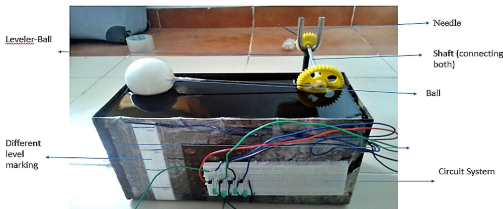
Fig 7: Demo of Proposed Water Level System
