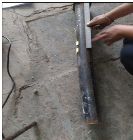
Figure No. 3 Deformed Circular CFST Columns after Experiment
