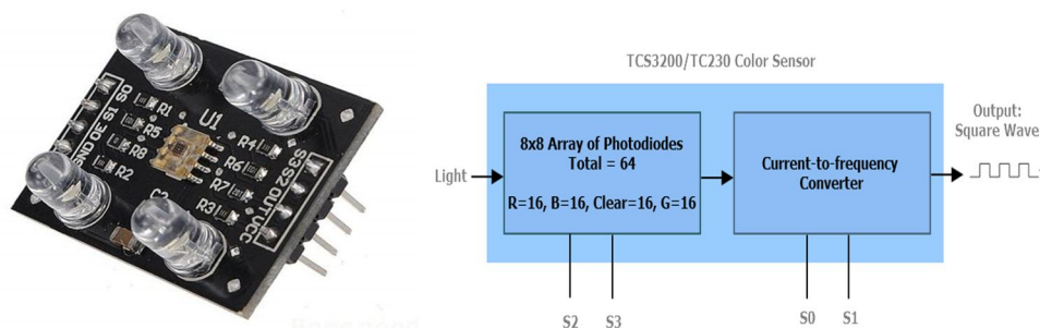
Figure 2: TCS3200 Colour Sensor
