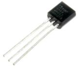
Temperature sensor is a gadget which detects varieties in temperature crosswise over it. LM35 is a fundamental temperature sensor that can be utilized for test reason. It give the readings in centigrade (degree Celsius) since its yield voltage is directly relative to temperature. It utilizes the way that as temperature expands, the voltage crosswise over diode increments at known rate (really the drop crosswise over base-producer intersection of transistor)
