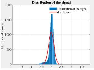
The .wav signal is processed by MATLAB software. First histogram analysis is performed for distribution of the signal which classify the intensity level and we can get the quality measure of the fruit
