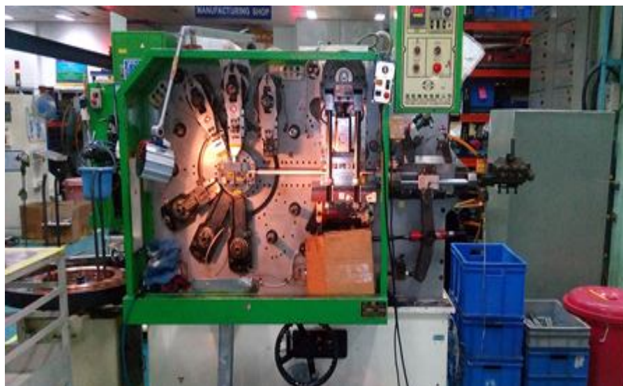
Fig 6: YSM Multislide Machine With Press Tool
