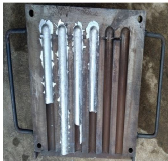
Fig – 2: Mould for specimen casting
