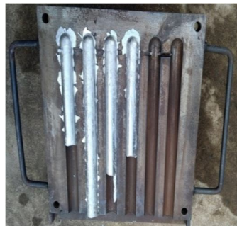
Fig – 2: Mould for specimen casting
