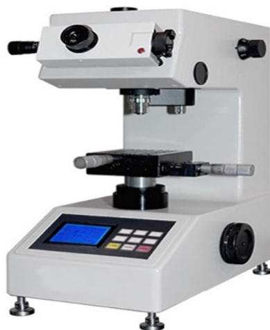
Fig – 6: Micro-vickers hardness equipment
