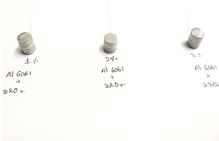
Fig – 7: Hardness testing specimens
