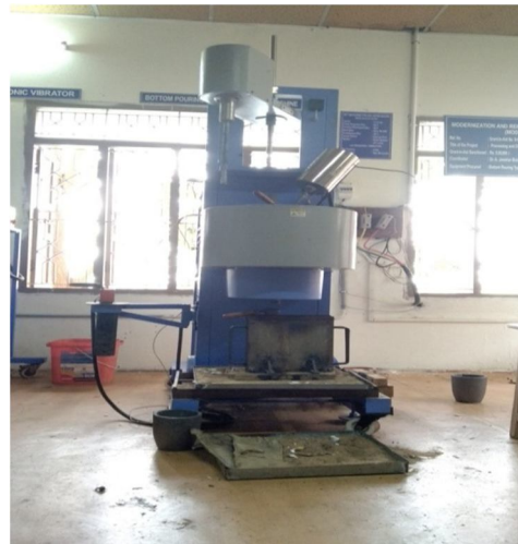
Fig – 1: Bottom pouring stir casting machine
