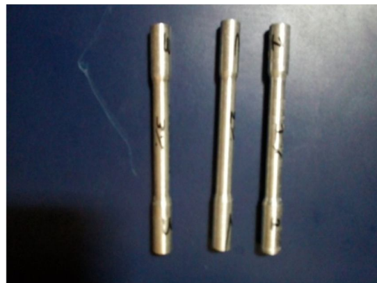
Fig – 4: Tensile strength specimens
