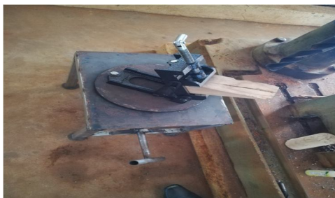
Fig. 3.3 Fabricated model of Rotating and Tilting vice
