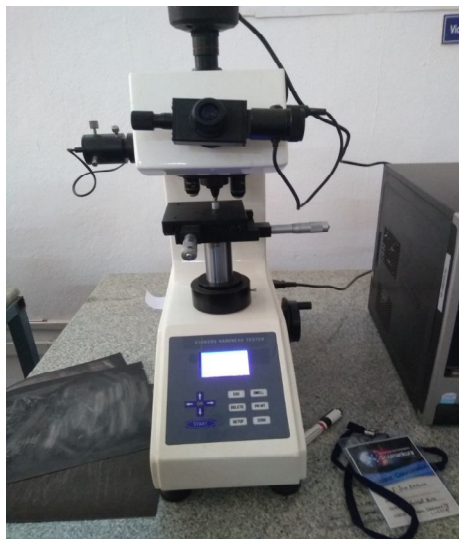
Fig – 8: Hardness measuring instrument.
