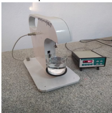
Fig – 7: Density measuring instrument.
