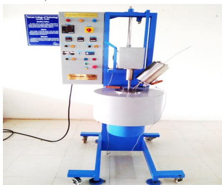
Fig – 4: Bottom pouring stir casting machine
