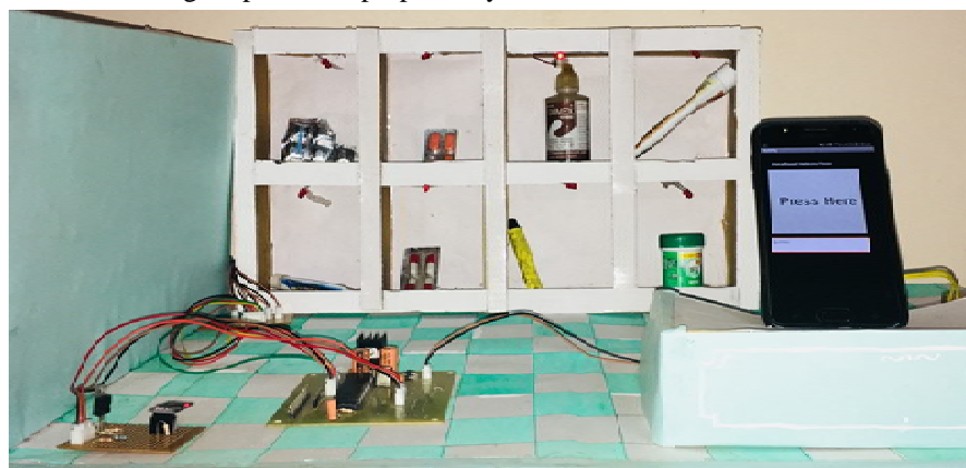
Fig. 3 Presentation model of ‘Medicine Locator’ containing Hardware, Medicine Compartments and Android phone.
