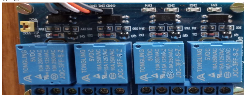
Fig. 7(i) Relay status after receiving Message
