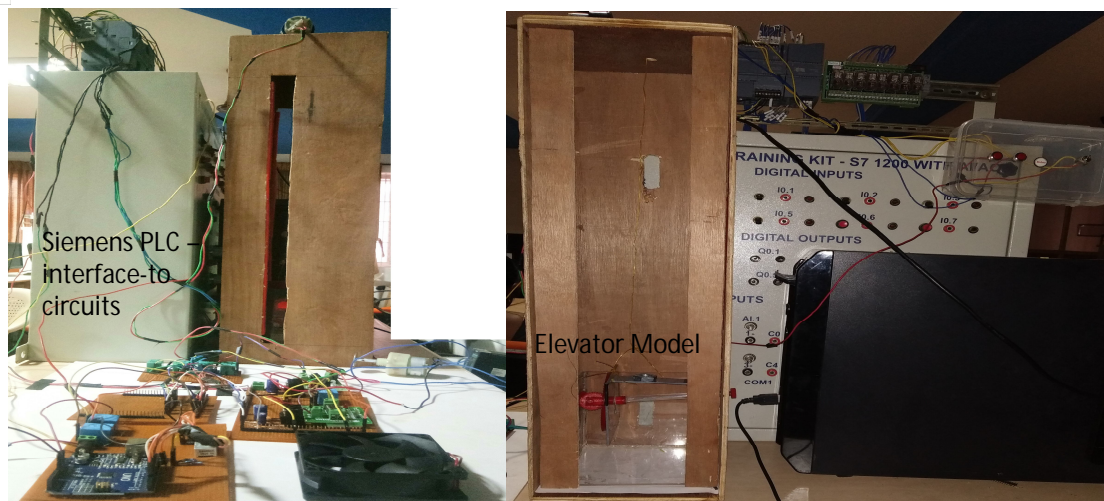
Fig.9 Interfacing of elevator with siemens PLC
