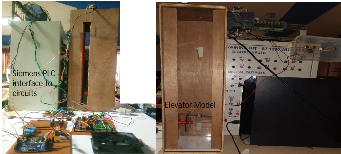
Fig.9 Interfacing of elevator with siemens PLC
