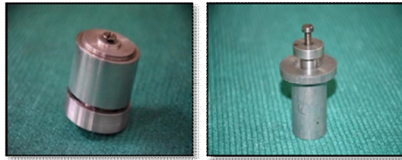
Fig 5: Microwave components holding fixture
