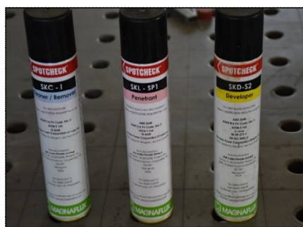
Fig 7: Cleaner, Penetrant & Developer of DP test
