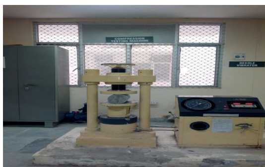
Figure 9: Split Tensile Strength Test by CTM.
