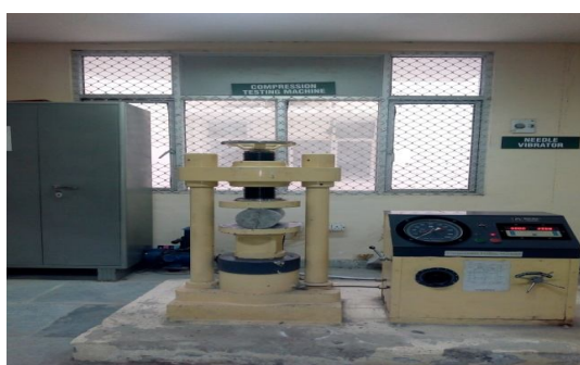
Figure 9: Split Tensile Strength Test by CTM.
