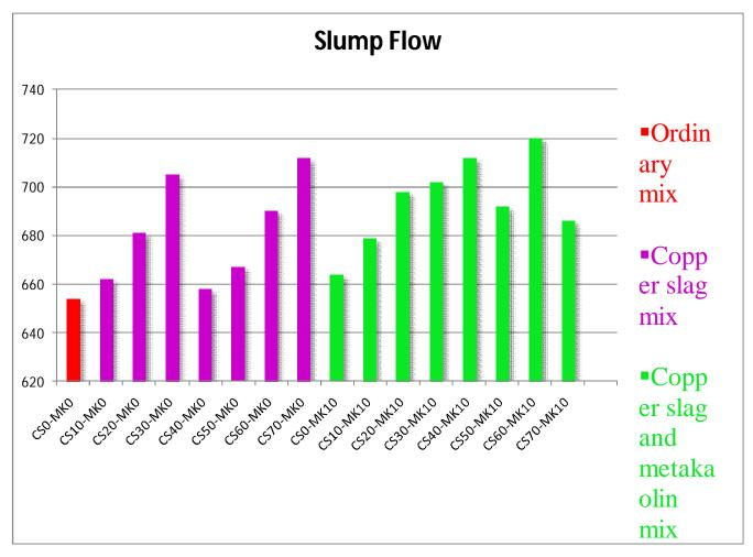
Slump Flow Test: From the Observation replacement of copper slag and metakaolin will improve the fresh properties of concrete. Optimum result for the slump flow test is being achieved with 70%CS and 0% MK and 60%CS and 10%MK. Increment of copper slag proportion will improve the slump flow of fresh concrete.
