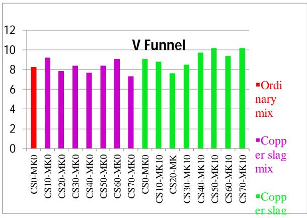
*3) V-funnel Test:* From the Observation optimum result for the v-funnel test is achieved from CS70%-MK0% and CS50%-MK10%. Higher replacement of Copper Slag improves the results for the fresh properties of self compacting concrete.
