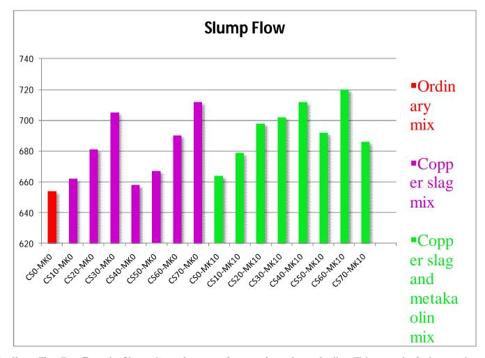
1) Slump Flow Test: From the Observation replacement of copper slag and metakaolin will improve the fresh properties of concrete. Optimum result for the slump flow test is being achieved with 70%CS and 0% MK and 60%CS and 10%MK. Increment of copper slag proportion will improve the slump flow of fresh concrete.
