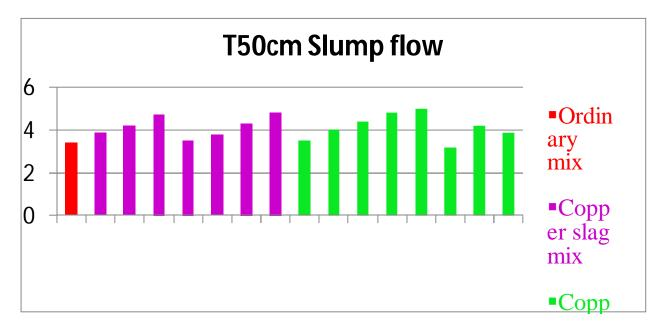
2) *T50 cm Slump flow Test:* From Observation T50 cm slump flow test results are being improved with slight increment of copper slag and Metakaolin. Optimum result for the test is achieved at CS40%-MK0% and CS50%-MK10%.
