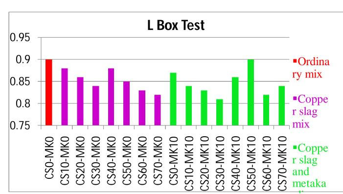
*L-box Test:* This test is very important for the checking of flow of self compacting concrete. Optimum result is achieved by replacement of CS70%-MK0% and CS30%-MK10%.
