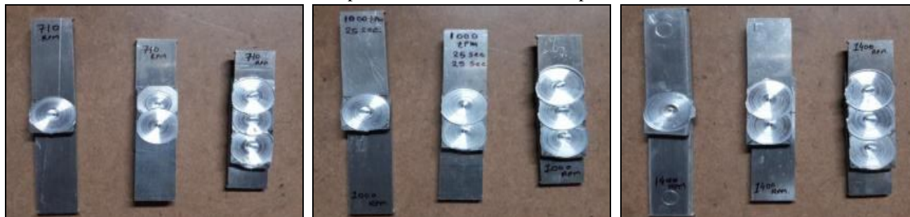
Fig.5 FSSW plates at 710RPM, 1000RPM and 1400RPM
