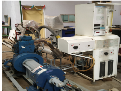
Fig. 6 Computerized variable compression ratio test rig.
