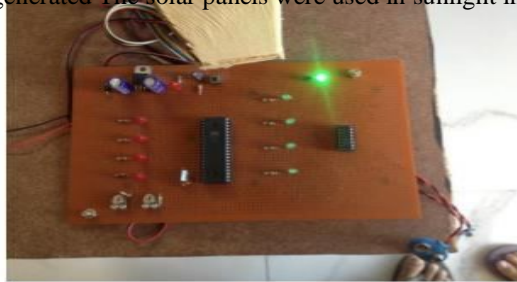
Fig. 3 Sun Tracking Solar Panel Hardware
