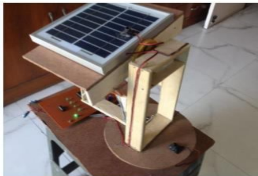
Fig. 2 Complete Hardware Module of Sun Tracking Solar Panel
