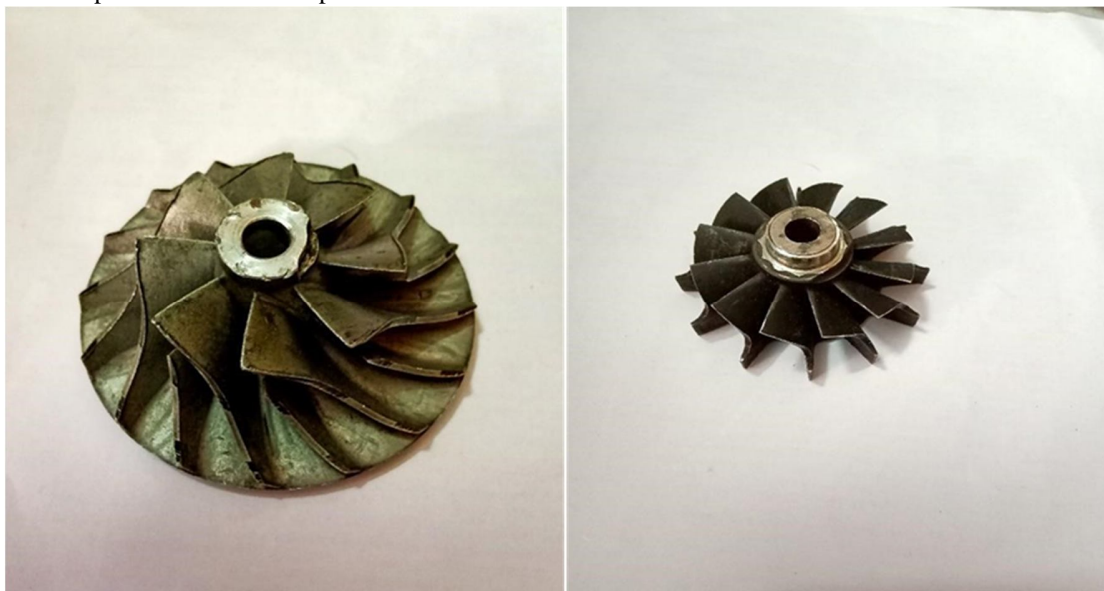
Fig. 8 Compressor And Turbine parts from the turbocharger
