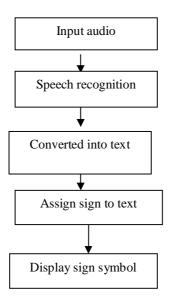
So in this architecture user give the audio input into computer, then this audio input is passed to speech recognition, speech recognition converts that audio into small understandable pat of text, speech recognition used different technology to break down the audio into text.
