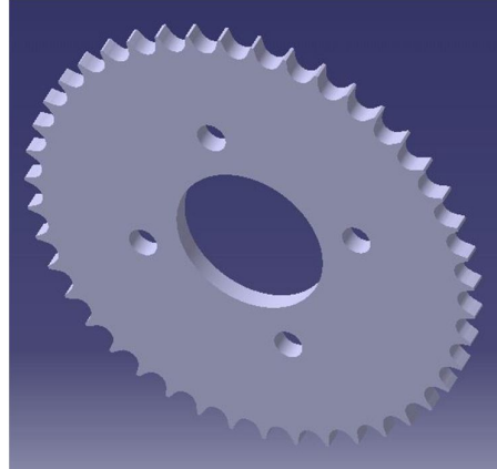
Fig. 5 3D model of sprocket
