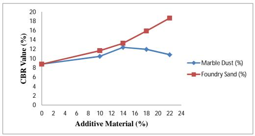
The study concludes the CBR percentage of soil with addition of Foundry Sand. On addition of Foundry Sand, the CBR value goes on increasing which signifies that the strength goes on increasing.
