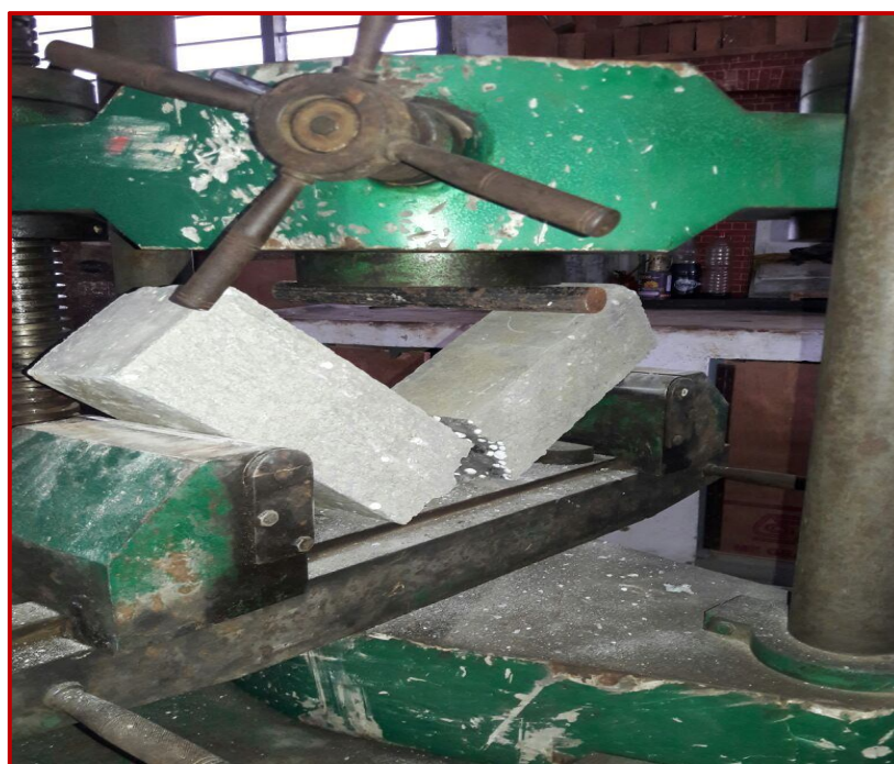
Fig.9 failure of flexural strength test
