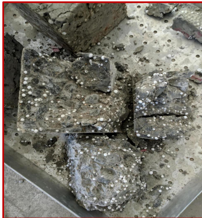
Fig. 5 failure concrete cube
