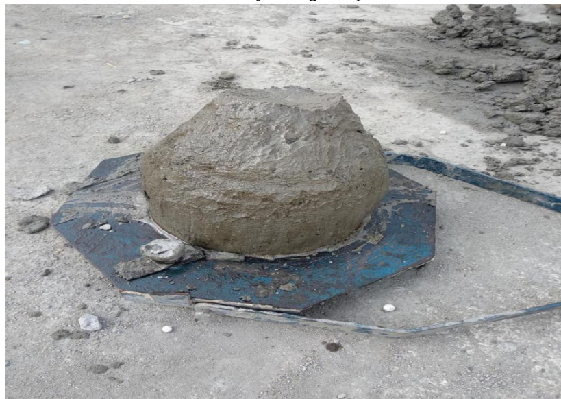
Fig. 3 slump cone result
