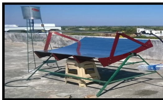
Experimental setup of parabolic solar trough collector with magnifying glasses
