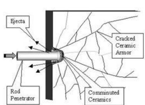
Fig. 1: Process of projectile penetrating the ceramic armor
