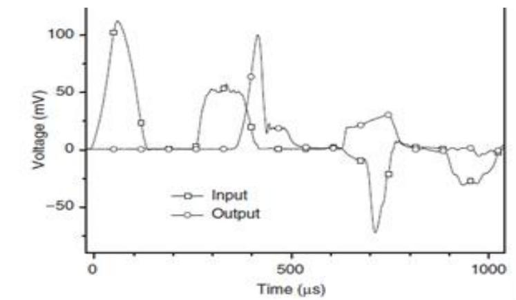
Fig. 8: typical oscilloscope trace of double pulse SHPB
