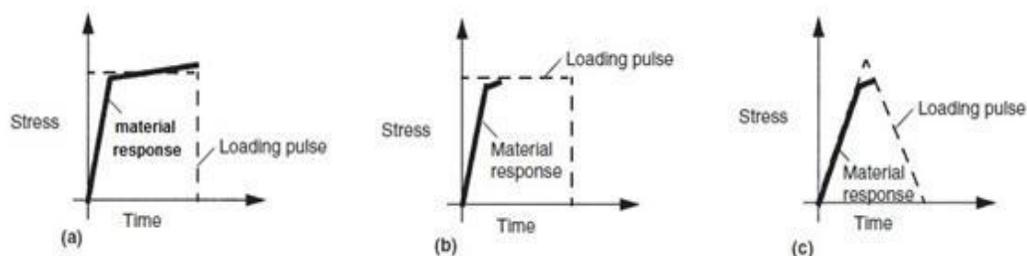
Fig. 6: illustrate the ceramic response and loading pulse
